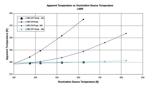
Figure 18: LWIR Apparent Temperature vs. Illumination Source Temperature
