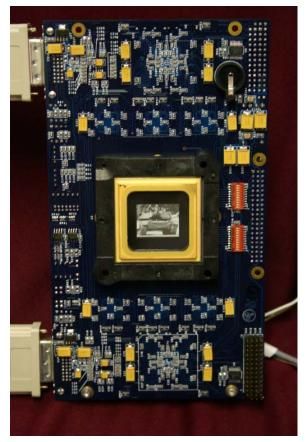
Figure 13: SXGA Drive Electronics & DMD
