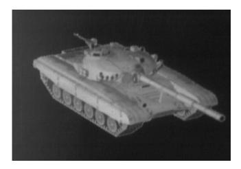
Figure 21: LWIR SVGA Collected by 320x240 Uncooled Bolometer Array Camera
