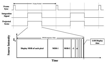
Figure 7: Synchronized PWM Timing
